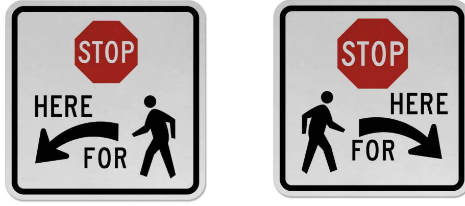
PEDESTRIAN CROSSING SIGN DETAIL N.T.S.
